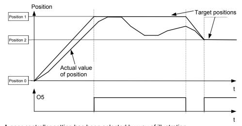
A poor controller setting has been selected by way of illustration.
